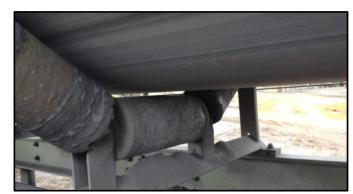
Conveyor lifting off old weigh-area
