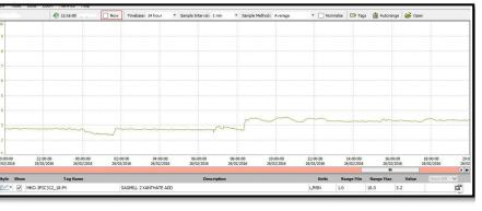
A trend screenshot from the DCS of the reagent process variable (with no set-point changes) when the existing GEMU valve was used.
