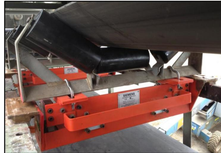
New MMI Frame Installation with balanced and adjustable rollers
