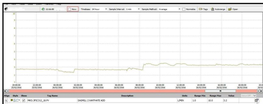
A trend screenshot from the DCS of the reagent process variable (with no set-point changes) when the existing GEMU valve was used.
