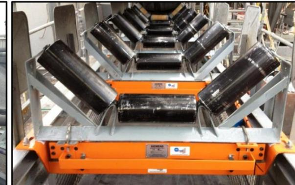
*New MSI frames fitted and aligned*
