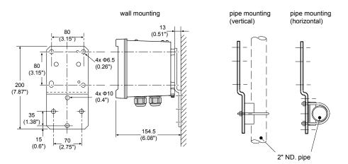
(Note)When option code "/UM" is specified, universal pipe/wall/panel mounting kit are supplied---same as option code "/U" and "/ PM" both specified.
