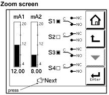
The zoom screen displays an easy graphic representation of the output functions. When "Next" is pressed it will give access to the logbook data.
