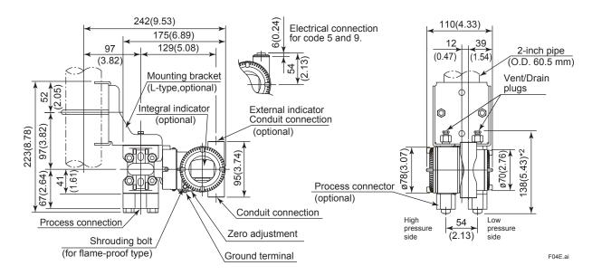
• Horizontal Impulse Piping Type (INSTALLATION CODE '9') (For CODE '8', refer to the notes below.)
